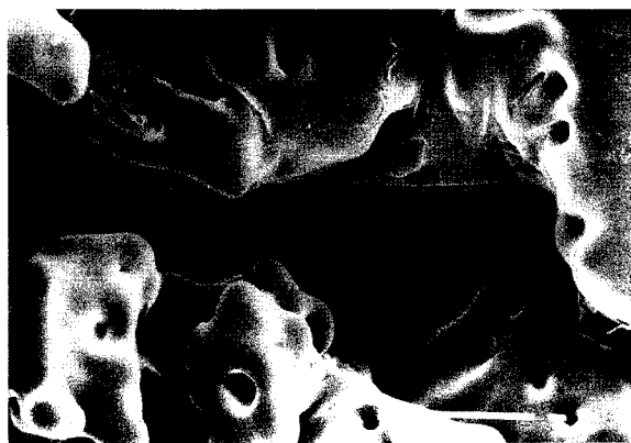
Fig. 4. Scanning electron micrograph for crystalline compound heated to 150°C and cooled to 30°C. 2000×; reduced 40% for reproduction.
